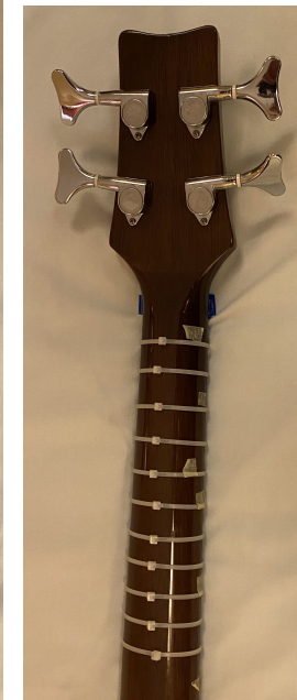
Figure 8. Refretted guitars. a) Hans-Gunter Lock's Thomann classic guitar refretted by Timo Tuhkanen (Finland), b) Gonzalo Muruaga Olguin with his electric 22-EDO guitar, neck refretted by Timo Tuhkanen c) a fretless acoustic bass guitar, experimental zip tie frets by Hans-Gunter Lock
